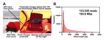
**Figure 3.** Two off-grid sequencing runs yielded almost 190 Mbp of data. (**A**) The solar power strategy for powering a laptop running Oxford Nanopore offline MinKNOW software (v18.12.9). Items shown are labelled. (**B**) Read length distribution for pooled sequencing runs. For simplicity only reads <5000 bp are shown.
